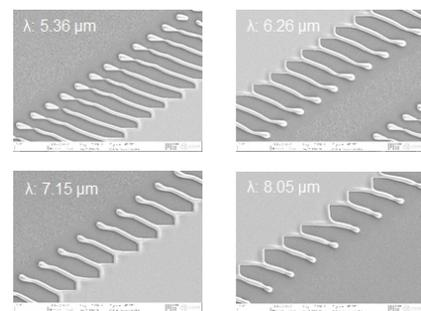
▲ Figure 2: Wires formed by templating a fingering instability using patterned periodic edge roughness.
