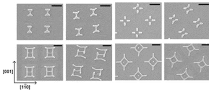
▲ Figure 1: Patterns formed by solid state dewetting of square patches of Ni films patterned with different sizes and crystallographic orientations.
